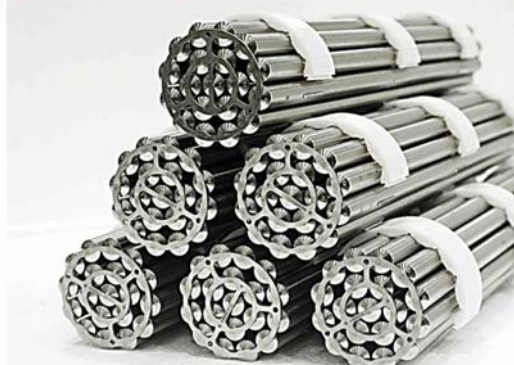
Zircaloy clad fuel bundles for PHWR
