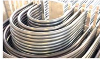
Heat exchanger tubes
